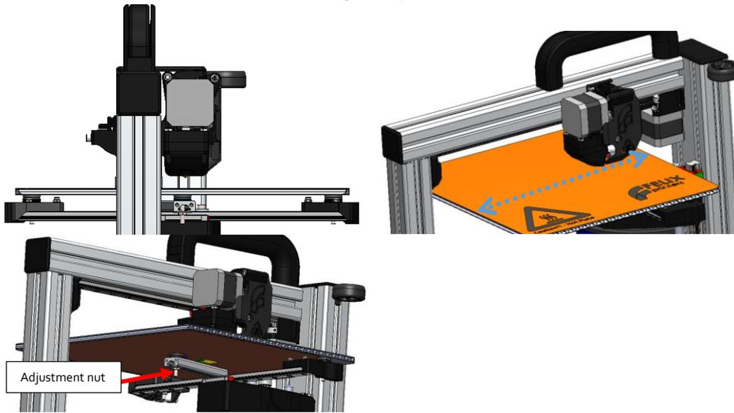
5. Move the X-axis carriage over its movement range slowly. While moving check the distance between the hot-end and bed. If the distance is not even, adjust it with the nut which supports the middle of the table.
