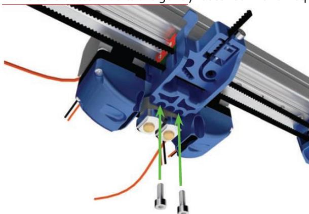
4. Is the height of both hot-ends equal? If not, do the following checks to see what could be the cause.
