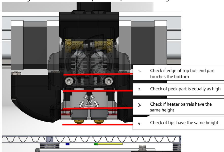
If there is a difference, it could be that the hot-end parts are not fastened equally between the hot-ends.
