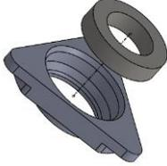
Break away the thin flange of the part below. (The flange was used to get better adhesion to the heated bed.)
