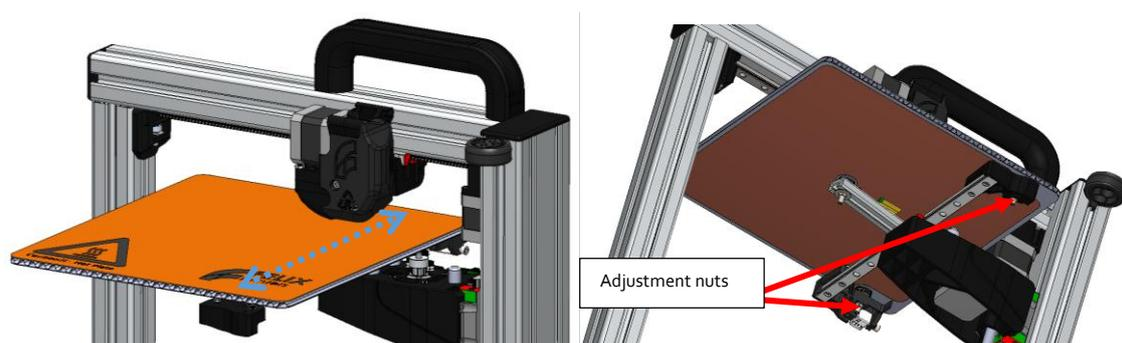
3. Move the table a little closer to the hot-end and repeat the previous step to more precisely determine the distance between the hot-end and the table over the whole length.
