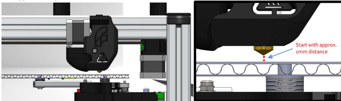
2. Move the Y-axis (heated bed) back and forth slowly. While doing this check the distance between the tip and bed while. It should be the same over the whole movement. If it is not turn the 2 screws underneath the bed as indicated in the picture below.
