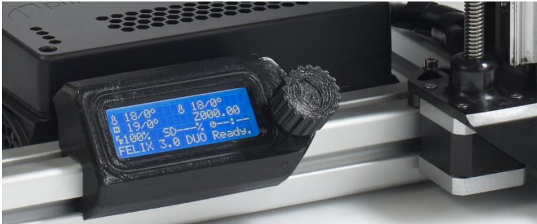
When in a menu in front of each line there will be a cursor, you can go down a line by rotating the rotary button. When you are at the line you want to be you can press the rotary button.
