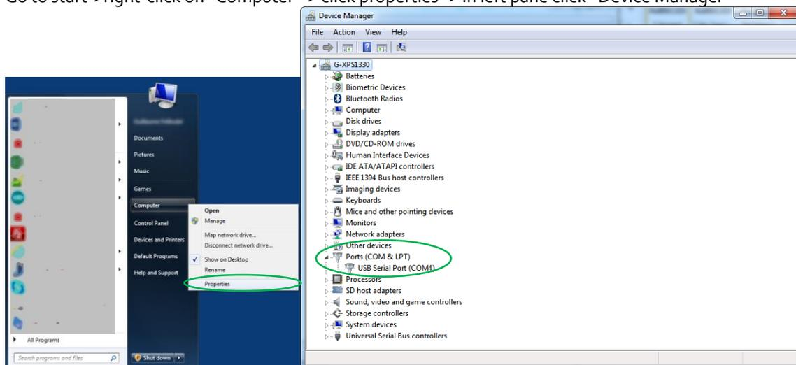
Note what COM-port is present. If there are more than one COM ports available unplug the USB cable of the printer, and re-plug it again. Check what port number is appearing and disappearing. This port number will be used for the next step.
