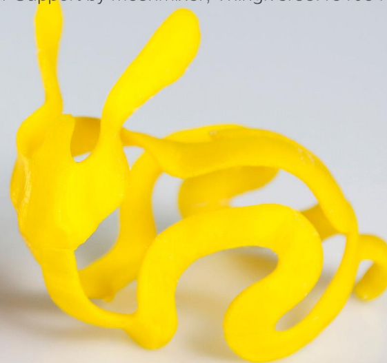
Dual Extruder Support Material Test: PLA&Support@0.15mm Layer Height original Bunny Peel from Bunny Peel with meshmixer Support by meshmixer, Thingiverse:131054
