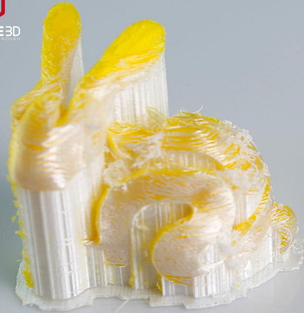
Dual Extruder Support Material Test: PLA&Support@0.15mm Layer Height original Bunny Peel from Bunny Peel with meshmixer Support by meshmixer, Thingiverse:131054
