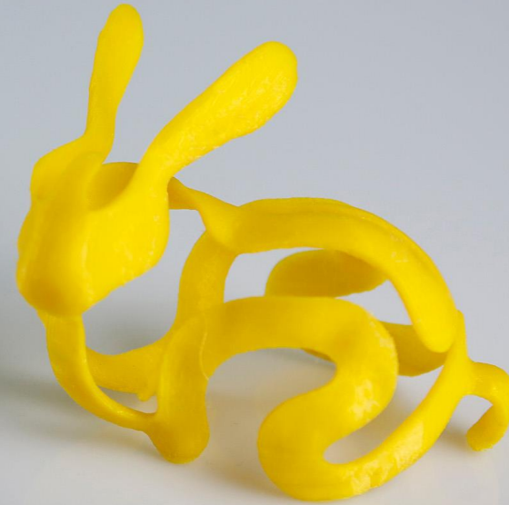
Dual Extruder Support Material Test: PLA&Support@0.15mm Layer Height original Bunny Peel from Bunny Peel with meshmixer Support by meshmixer, Thingiverse:131054
