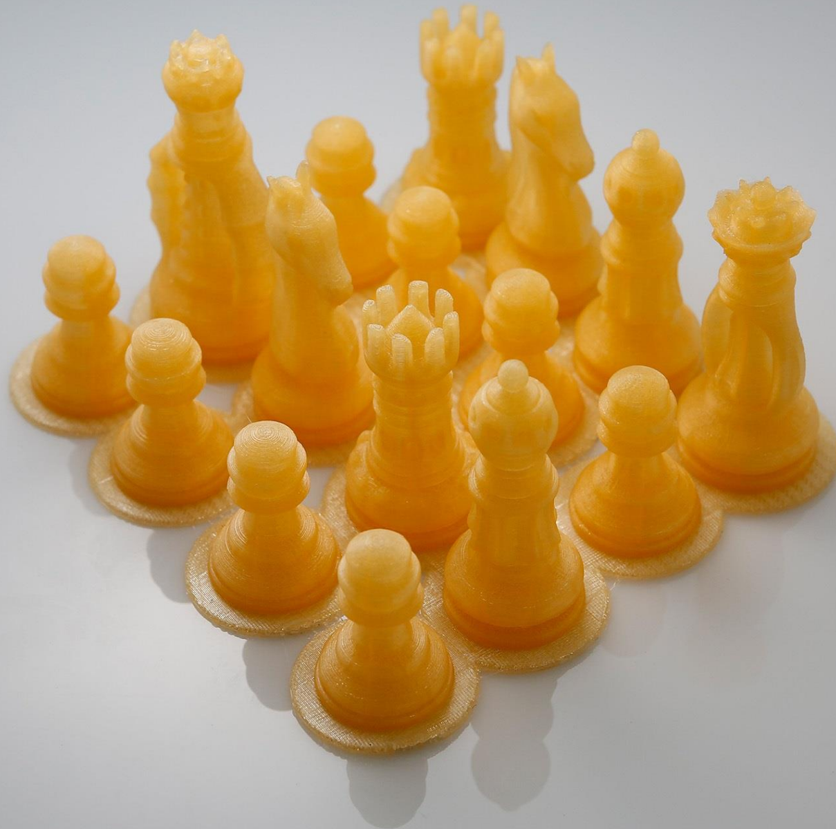
Multiple Object Print Test: PLA @0.15mm Layer Height with Raft unremoved Chess – Classic Set by by SteedMaker, Thingiverse:34017
